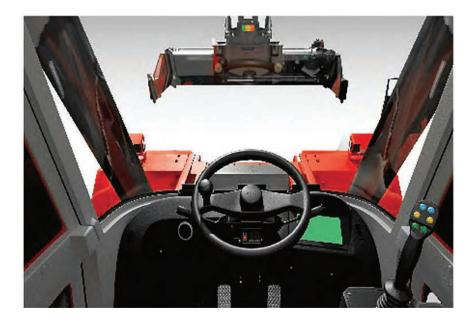
Cabin noise at the operator's ear level have been reduced to 70 dB
