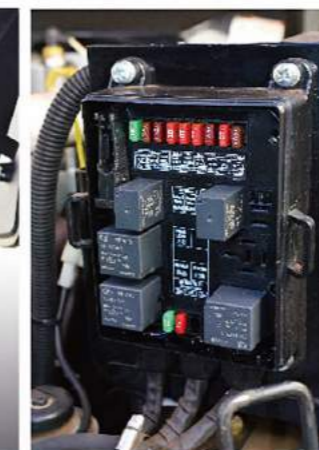
Modular high protection electrical box
