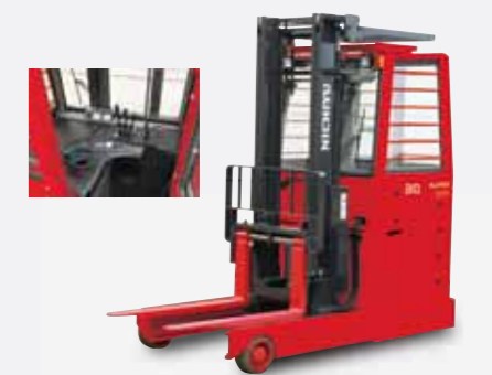
Fully cold-storage Specification (capsule forklift)
