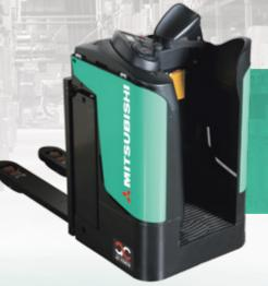
The ergonomic layout of the controls on the console contributes to smooth and easy operation. The comfortable operator's compartment has a cushioned backrest and suspended floor, an arm rest is optional.
