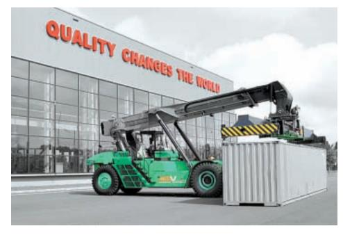
A Reach Stacker needs a quality spreader. The exceptional Elme 817 spreader is suitable for lifting both 20ft and 40ft containers with an impressive side shift of plus/minus 800mm.
